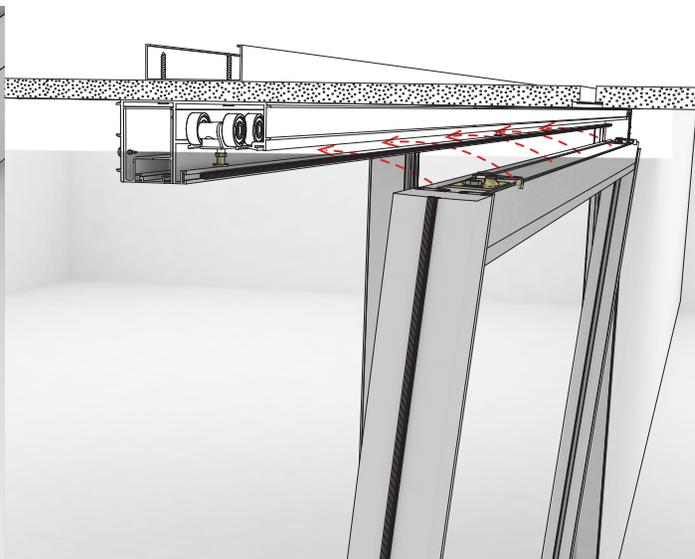
The sliding hardware is shipped installed in the track. Stops can be adjusted to the proper location using a phillips head screw driver.
